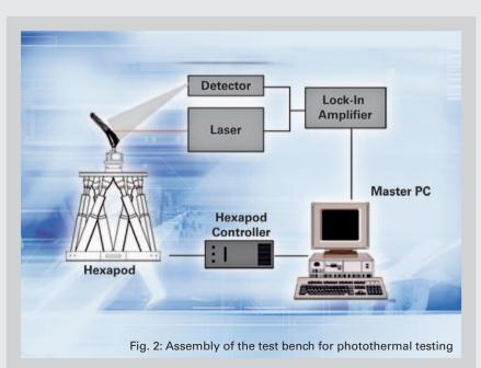
on arbitrary surfaces can be performed. The kinematics of this system consists a six-axis PI M-840 Hexapod (Fig. 1) which can be coordinated with various common machines such as industrial robots or machine tools. Test samples used included medical implants.
